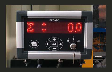
This function automatically **opens-up the minimum and maximum limits** when the press stops. Upon re-starting the limits are then gradually closed back to their *original values*. This allows tighter limit setting when the press is running giving **better press protection**.
