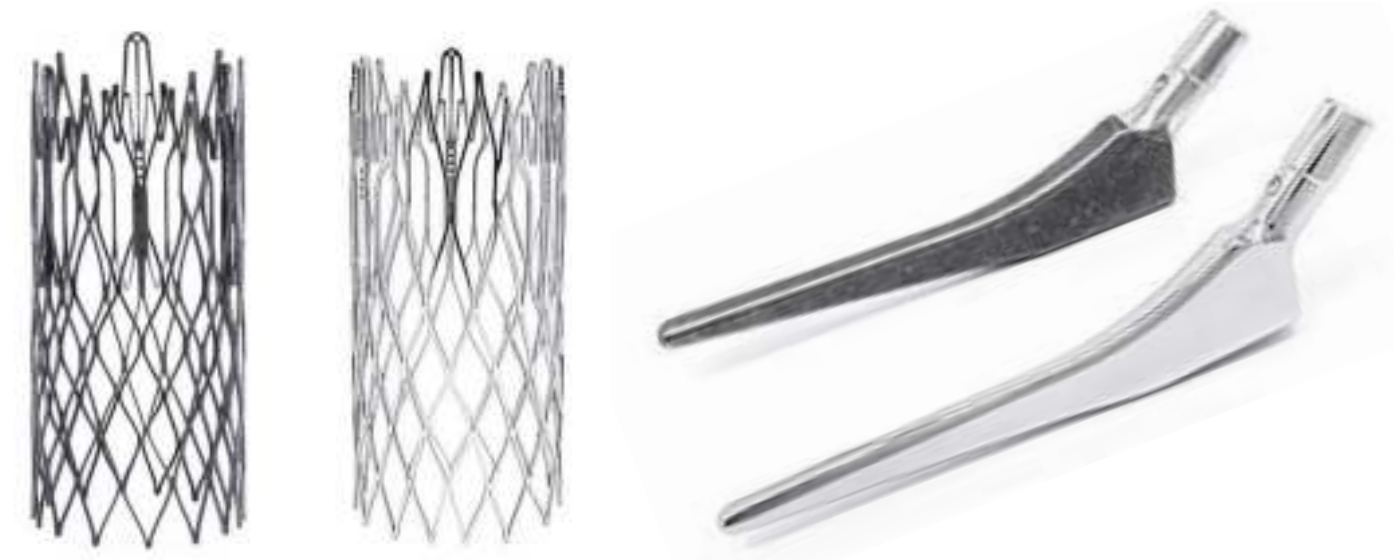
Ra: 0.09 µm (after the dry electropolishing process)
