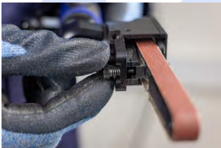
In a clockwise motion, use the smaller locking screw to lock the desired position in place
