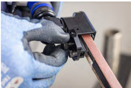
Using the larger adjustable tracking screw, rotate until desired position of belt is established
