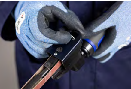
Remove the safety guard by pulling the safety catch towards you
