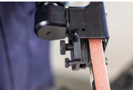
Run the tool with the belt attached, noticing any slippage or run out on the belt
