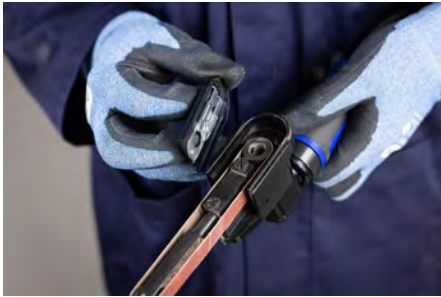
Once the guard is removed, replace the abrasive belt
