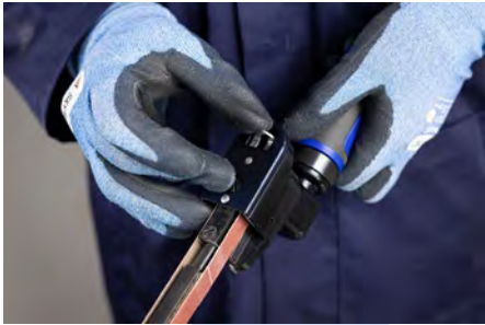
Place the guard back onto the tool and push the safety catch to engage with clasp
