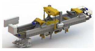
Stretch forming machines for sheets are designed to meet all tonnage, length, and width specifications. These machines have been widely used in stretch forming aluminium fuselage, wing, and engine cowl panels. Still, the process has now evolved to forming exterior panels on a high-speed locomotives, recreational vehicles, and buses, as well as proprietary aerospace and commercial rocket applications.
