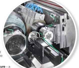
Tschudin's Proline series benefits further from **another patented feature** – a fourth CNC Y-axis that moves the regulating wheel vertically in order to **remove the need for an operator to adjust the workrest blade height** to keep the grinding geometry consistent as the grinding wheel wears. As this innovative feature is linked to the CNC programme, the regulating wheel height is moved automatically. **Natural granite machine** beds offer maximum
