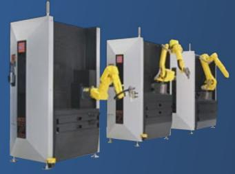
Fanuc or Staubli 6-axis robots are used for handling parts from 1g up to 700 Kg in weight. These are very versatile systems and are suited for loading a huge variety of machines of all types and applications. Various component storage solutions are available including the use of pallets, conveyors, rotary tables, data matrix code reader/writers and special one-off solutions.
