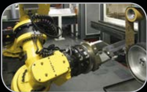
DEBURRING RAW BLADES BEFORE THE MECHANICAL PROCESSES
