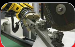
CUTTING RAW BLADES FROM THE MICROFOUNDED CLUSTERS
