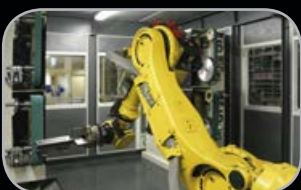
GRINDING AND FINISHING THE AIROFOILS
