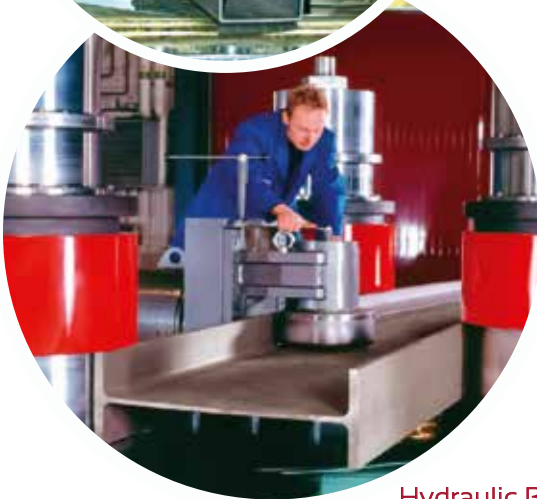
Hydraulic Beam on edge device ("pulling unit") R-15-S
