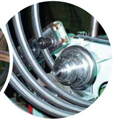
Half pipe spiral bending
